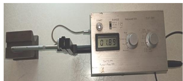
Fig. 6: Surface Roughness Experiment Setup
